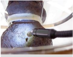
Underside of cascabel showing two holes, the upper is 8 mm in diameter, the lower is 4 mm. The smaller hole intersects with the larger just below the surface. The larger hole extends approximately 60 mm into the object. (Photo by ArtLab Australia, courtesy NT Heritage Branch)
