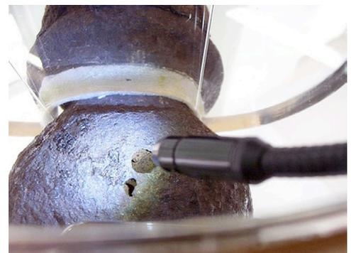
Underside of cascabel showing two holes, the upper is 8 mm in diameter, the lower is 4 mm. The smaller hole intersects with the larger just below the surface. The larger hole extends approximately 60 mm into the object. (Photo by ArtLab Australia, courtesy NT Heritage Branch)
